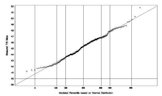
Vertical reference linee plotted at 1st, 10th, 20th, 50th, 80th, 90th, and 99th percentiles of fitted distribution Horizontal reference line plotted at spec minimum, 40 kel
