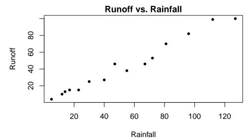
b) We fit a linear model with runoff as response and rainfall as predictor. We are then able to use this model for prediction.
