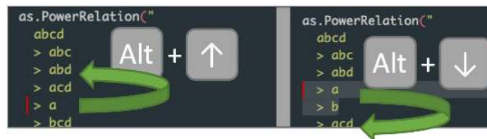
Figure 1: Using Alt+Up or Alt+Down to move one or more lines of code
