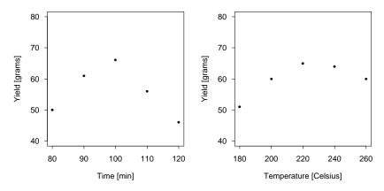
Left: Temperature  $T = 220^{\circ}C$  / Right: Reaction time t = 100 minutes.
