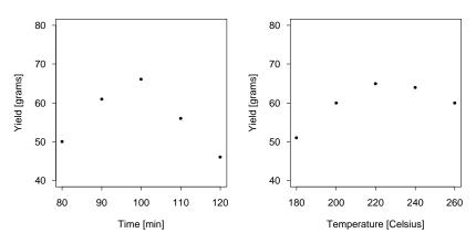
Left: Temperature  $T=220^{\circ}C$  / Right: Reaction time t=100 minutes.
